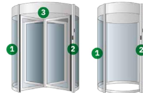
1. Door wing and curved sidewall glass: clear, poly-glass laminate, bullet-resistant, Level 3 glass (29mm thick)
